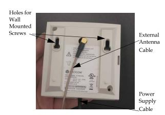
**Note:** The external antenna used for the transmitter is to be fixed-mounted on indoor permanent structures providing a separation distance of at least 20 cm/8 inches from all persons during normal operation and must not be co-located or operating in conjunction with any other antenna or transmitter. The maximum radiated output power is 1W e.i.r.p.
